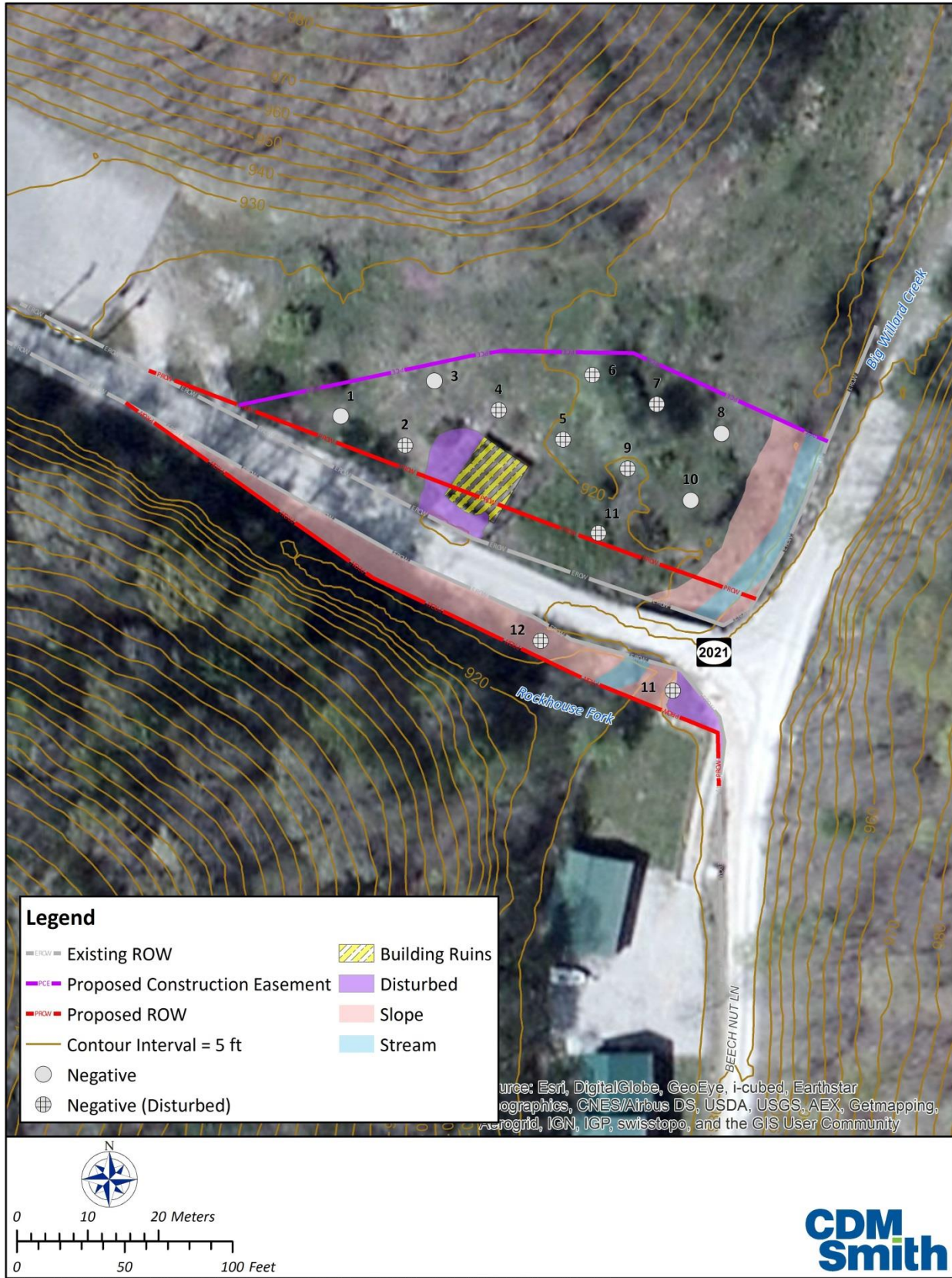
Figure 3-2. Location of SPTs on Aerial Photograph.
